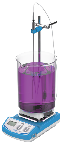
Magnetic stirrer to measure liquid temp.
